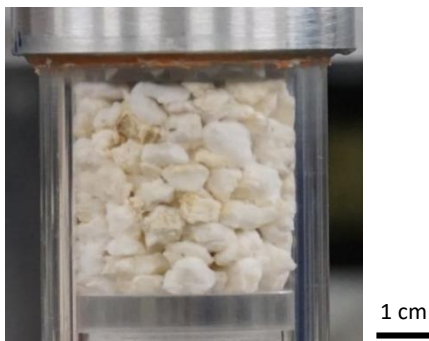
Figure 1 : Packing of sunflower pith particles (without compaction)
