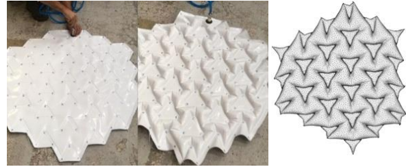
Figure 1 An inflated auxetic pad built at Navier and its finite elements simulation by Inria
