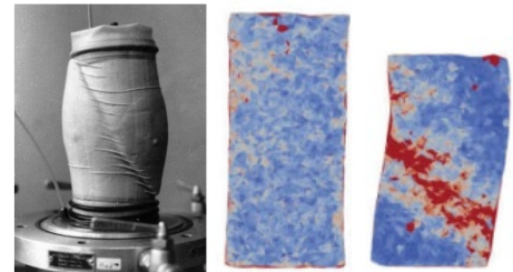
Fig.1: A shear band observed in a classical triaxial compression test (left); deviatoric strain field at different axial strain stages: \varepsilon_a = 3\% (middle) and \varepsilon_a = 12\% (right).
